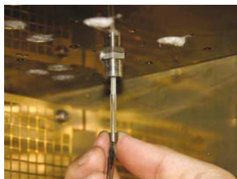
Simple nozzle replacement supports both capillary and packed columns.
