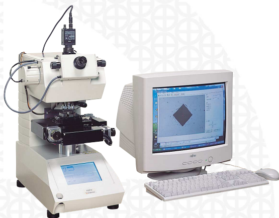
Full automatic micro Vickers hardness tester (Specimen attachment is option.)
